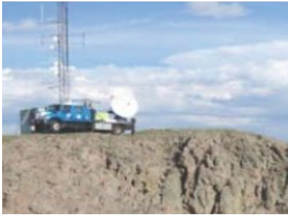
Doppler on wheels deployed during the late summer of 2013. Photo: Joshua Wurman, Center for Severe Weather Research
